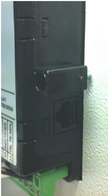
Installation of screw type bracket
