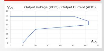
If the output power is below the nominal value, the unit will provide its nominal voltage. When the nominal power is attained the unit enters into power limiting mode and with an increasing current, the output voltage will decrease. When the maximum output current is reached, the unit will not provide more current and the voltage will drop. When the ouput voltage falls to 40V the unit starts reducing quickly its output current. The short circuit current is limited to 10Amps.
