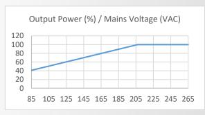
If the supply voltage goes below 207VAC, then the unit will limit its input current to 15.0Amps.
