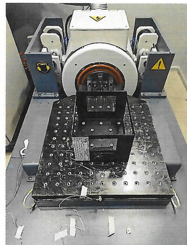
PICTURE 5.2 : After X Axis Vibration Test
